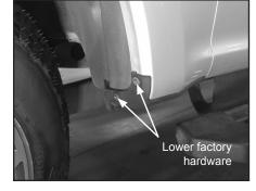
B. Align mud flap bracket holes with holes on mud flap. Then install with (2) 7mm screws through 3<sup>rd</sup> and 5<sup>th</sup> holes into newly free holes in wheel well. Use 7mm socket to start screw into mud flap.
