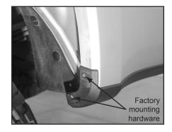
B. Align mud flap bracket holes with holes on mud flap. Then install with (2) #10 x 1-1/2" truss head screws through 2<sup>nd</sup> and 4<sup>th</sup> holes into free holes in wheel well. Secure with serrated flange nut and finger tighten.
