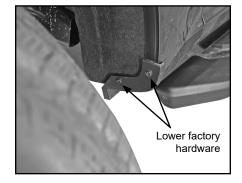
B. Align mud flap bracket holes with holes on mud flap. Then install with (2) 7mm screws through 2<sup>nd</sup> and 4<sup>th</sup> holes into newly free holes in wheel well. Use 7mm socket to start screw into mud flap.
