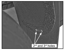
C. Install 5/16" x 1" Allen button head bolt through 1st hole in mud flap bracket, then mud flap. Holding bracket in place, insert clinch bracket behind mud flap and install onto 5/16" x 1" Allen button head bolt. Ensure clinch bracket is behind lip on wheel well with extended threads facing away from mud flap. Push clinch bracket as far behind lip as it can go. Leave bolt loose for now.
